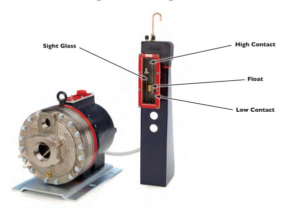
The Hydra-Cell Oil Level Monitoring Kit uses a Murphy SWICHGAGE Model L129CK1, which is field-proven to detect the crank case oil levels and is well-suited to detect oil levels for Hydra-Cell pumps except the F20, P100, T100, and Q155 Series models. (D35 shown)
