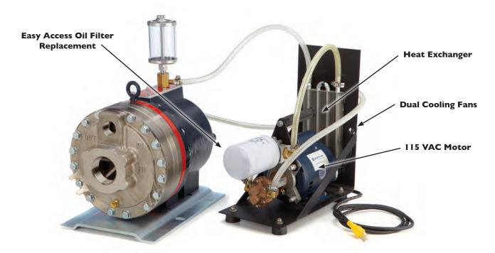
Hydra-Cell Oil Cooler and Filter Systems enable Hydra-Cell pumps to operate cooler in order to extend oil life and reduce bearing wear. This helps maximize performance and reliability in some of the toughest industrial and process applications. They are easy to install and available with all Hydra-Cell models except the F20, P100, T100, and Q155 Series models. (D35 shown)
