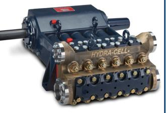
Pump Model: Q155ERDGHFEHAY x 2 Flow: 4000 BPD (117 gpm; 442 l/min) per pump Pressure: 600 psi (41 bar) Application: LACT system for transferring crude oil from an oilfield to a midstream pipeline
