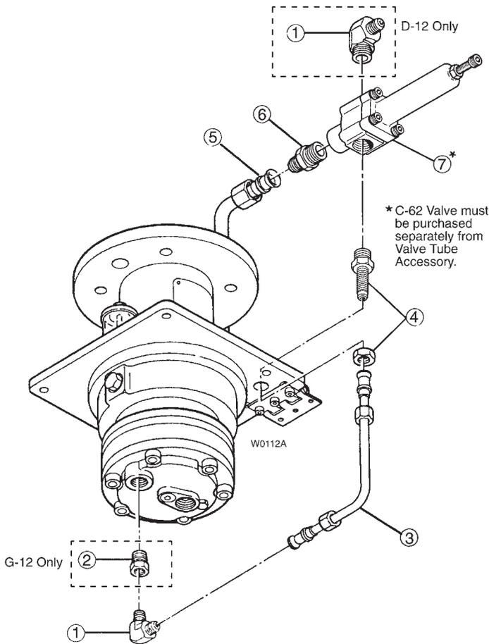
The Valve/Tube Accessory can be installed on either the right or left side of the pump housing.
