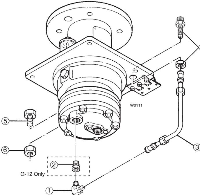
The Tube Accessory can be installed on either the right or left side of the pump housing.
