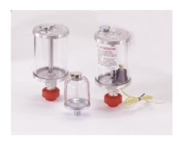
Oil reservoir assemblies easily screw in where the oil fill cap is located on all Hydra-Cell pump models D/G-O3 and larger. Pumps equipped with an oil reservoir provides more volume for oil expansion and allows for quick visual monitoring of the oil level and its condition.
