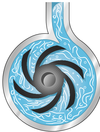
Typical Volute-Type Centrifugal Pump showing excessive turbulence and eddies
