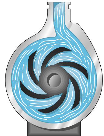
STAN-COR Concentric Casing Pump showing smooth flow pattern
