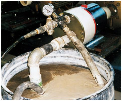
Pumping ceramic slurry at 40% solid content.
