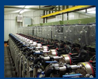
Enhanced oil recovery - pumping shear-sensitive polymers
