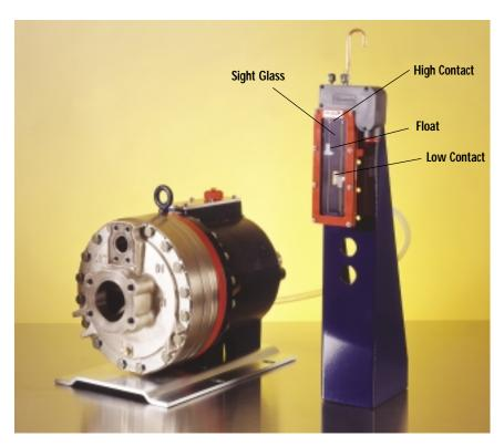
The Hydra-Cell Oil Level Monitoring System utilizes a Murphy SWICHGAGE® Model L129CK1. Field proven in the oil industry to detect crank case oil level, the Murphy SWICHGAGE is well suited to detect oil level for Hydra-Cell pumps such as the D/G-35 shown here.
